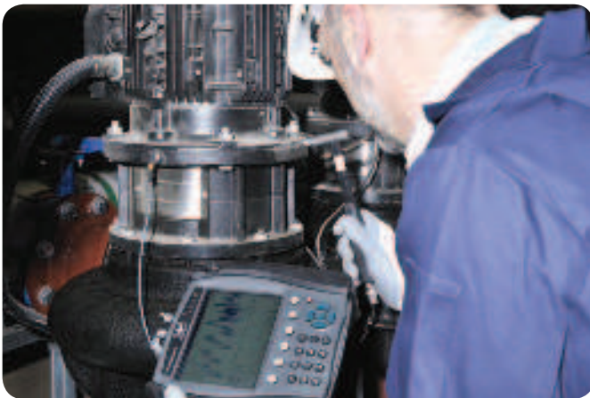
SKF Microlog AX provides fast data collection and analysis. The large screen facilitates viewing in any light.
